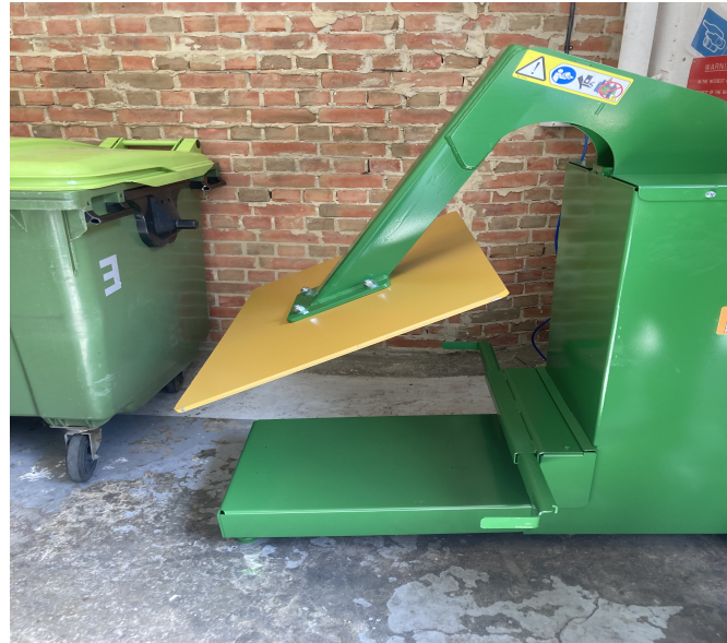
Picture 2. The position of the plates when not in use
